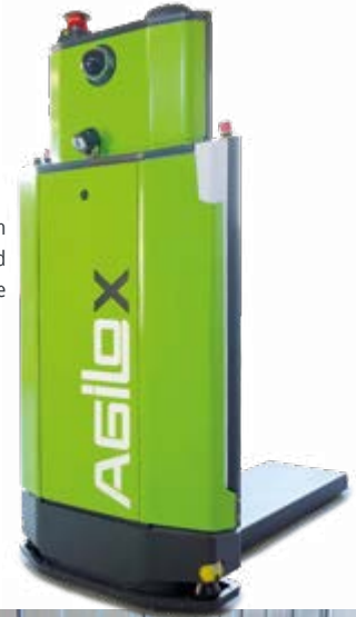
AGILOX NFK with obstacle avoidance and signal light package
